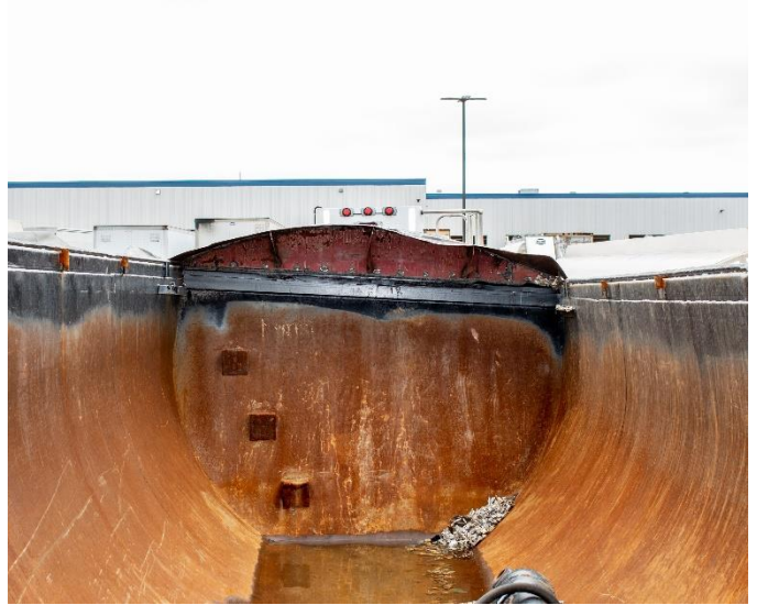
Figure 10 – Bent Trailer Frame
