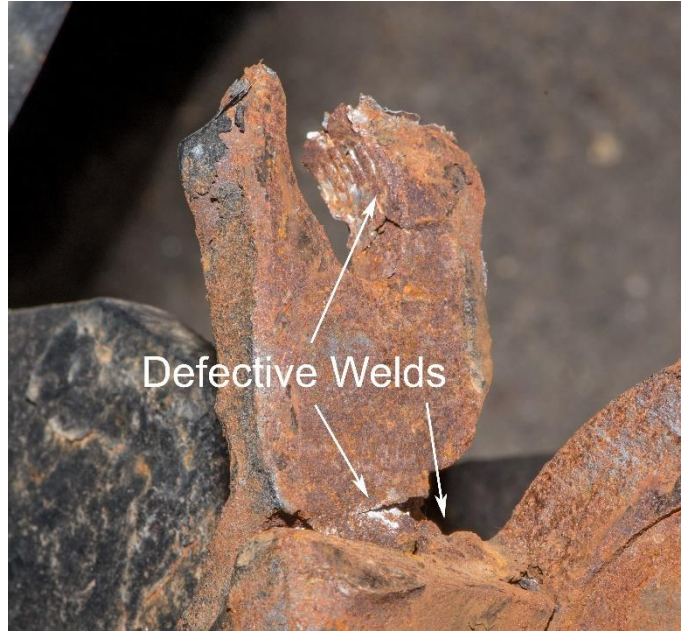
Figure 6 – Defective Welds Right Side - Rear Connection Bracket
