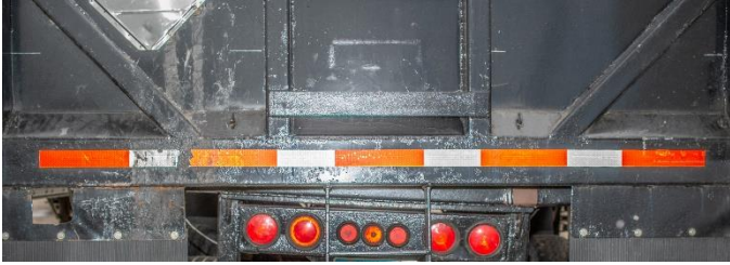
Figure 9 – Bent Trailer Frame
