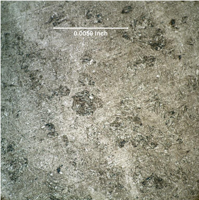
Figure 7 – 400X Sample 2 Microstructure
