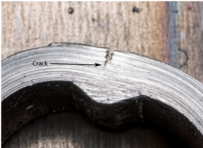
Figure 5 – Sample 1 Bend Test 1
