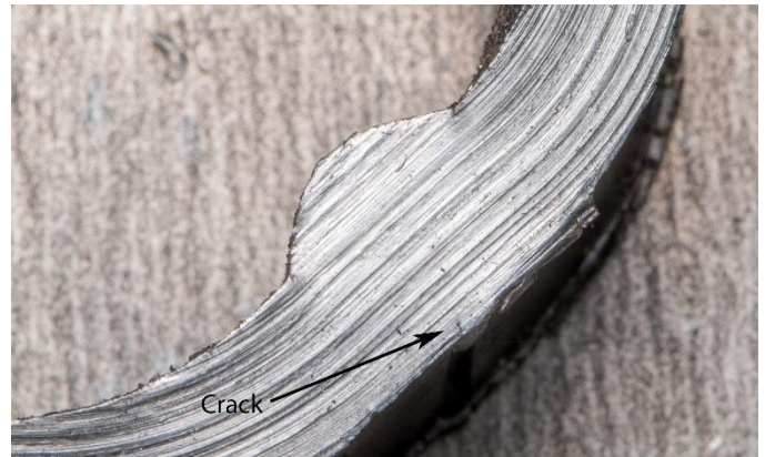
Figure 6 – Sample 1 Bend Test 2
