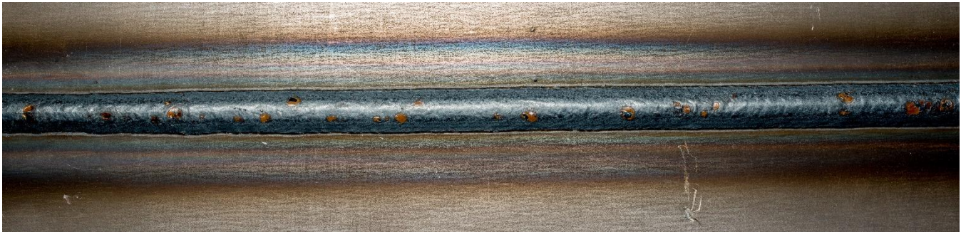
Figure 1 – Sample 1 CO 2 Cover Gas - Top Side
