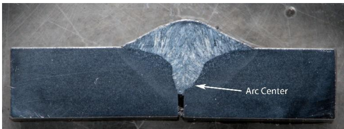
Figure 9 – Macro of Weld – Sample 1
