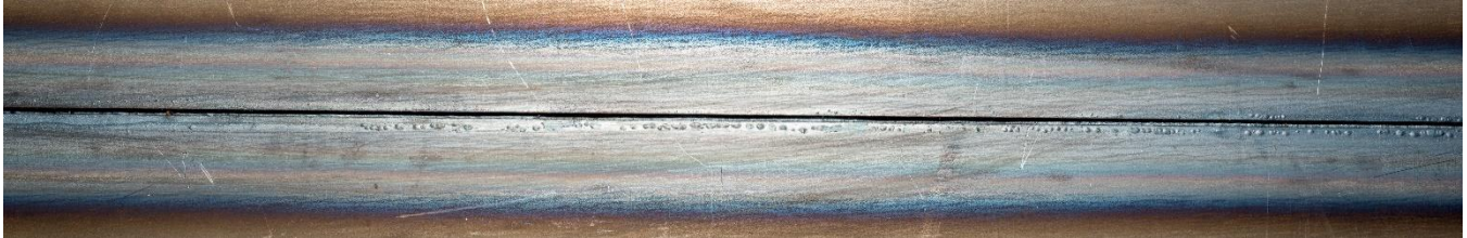
Figure 4 – Sample 2 Root Pass
