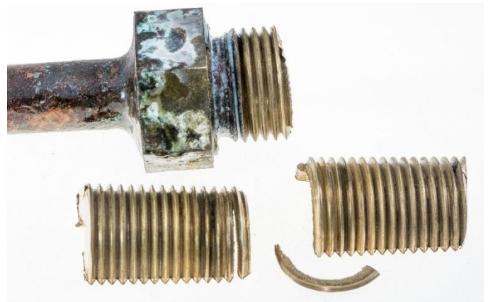
Figure 2 – Fitting 1 after Sectioning
