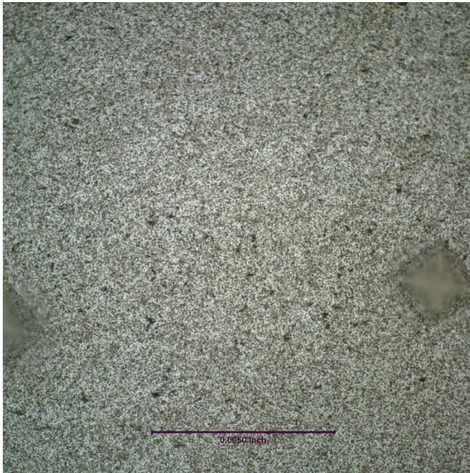
Figure 10 – 400X Microstructure of Stator Contact
