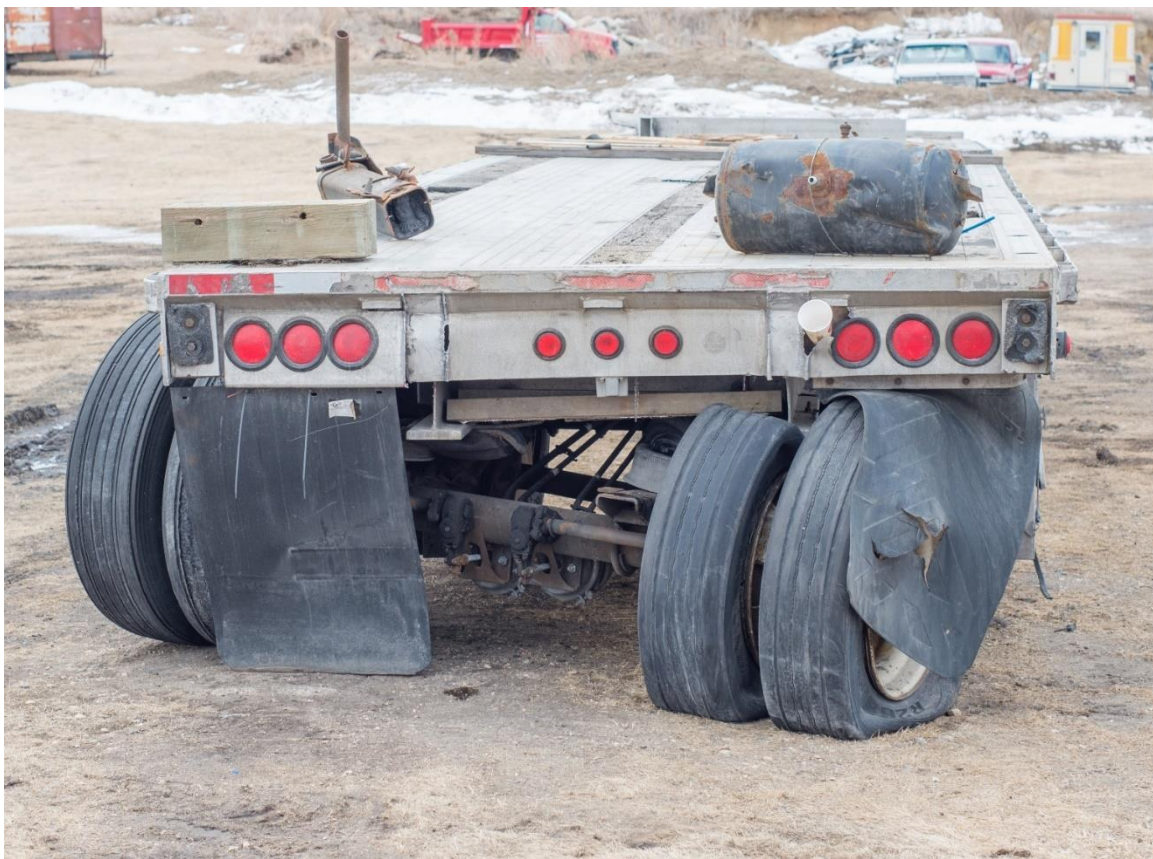
Figure 6 – Damage Shown from Rear of Trailer
