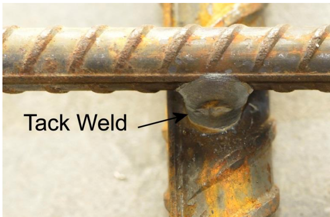
Figure 5 – Tack Weld, Exemplar 2
