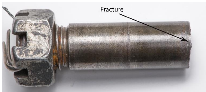
Figure 1 – Broken Coupler Pin
