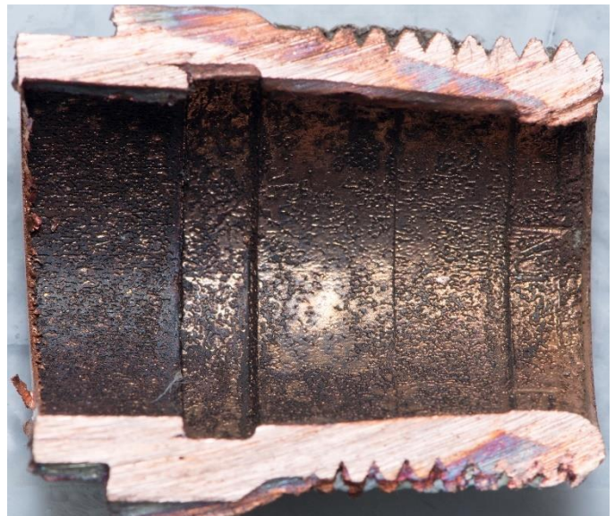
Figure 2 – Fitting after Sectioning
