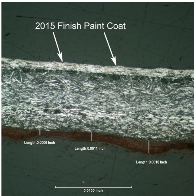
Figure 18 – 200X Cross Section - Paint Sample 1
