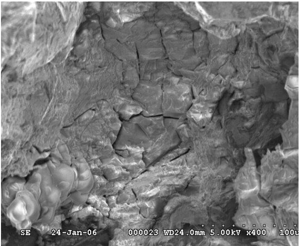
Figure 6 – 400X Intergranular Porosity
