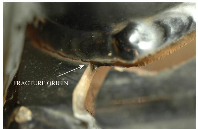
Figure 2 – Fracture Origin - Axle Housing Segment
