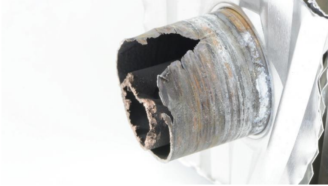
Figure 28 – Leak in Coil Sample 2
