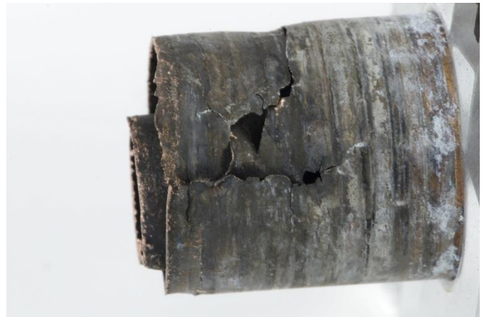
Figure 23 – Leak, Coil Sample 1
