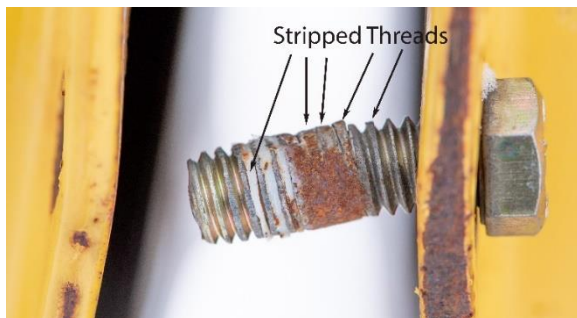
Figure 10 – Stripped Threads on Flange Bolt
