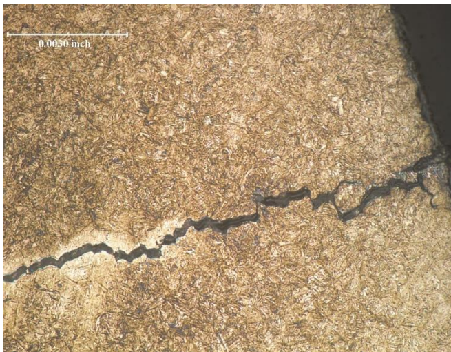
Figure 7 – 400X Intergranular Fracture and Case Microstructure
