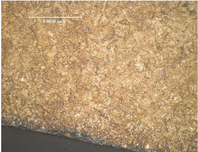
Figure 5 – 400X Tempered Martensite Case Sample 1
