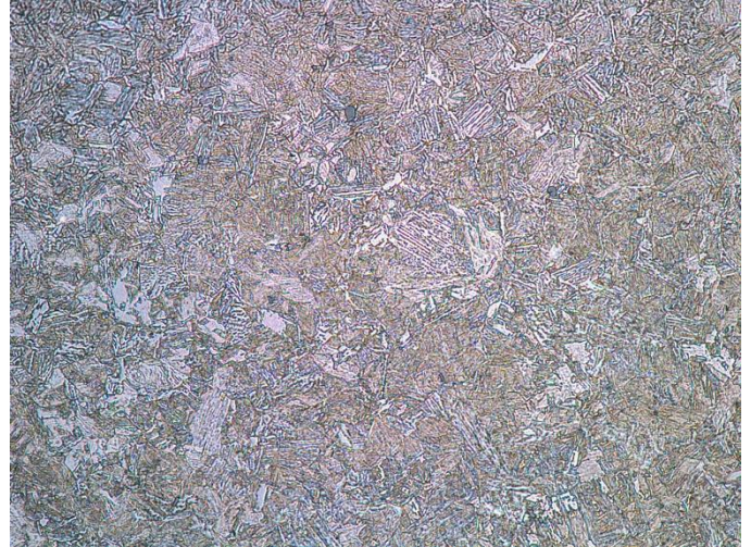
Figure 7 – 400X Microstructure Core of Shaft
