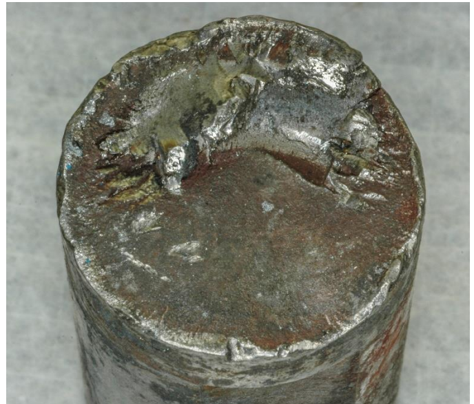
Figure 2 – Fracture Surface of Shaft
