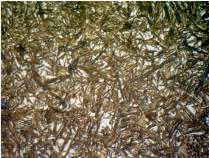
Figure 3 – 1500X Retained Austenite, Good Axle Bearing Surface
